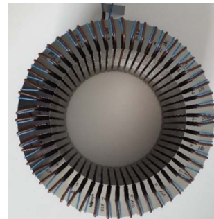
Fig. 1. Stator core with wound primary and secondary coils.
