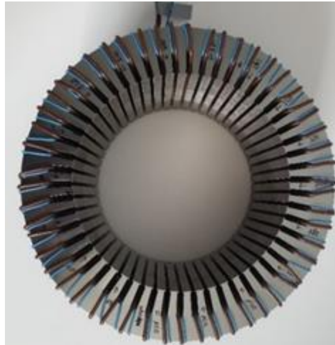
Stator with BST-M measurement coils wound on back iron
