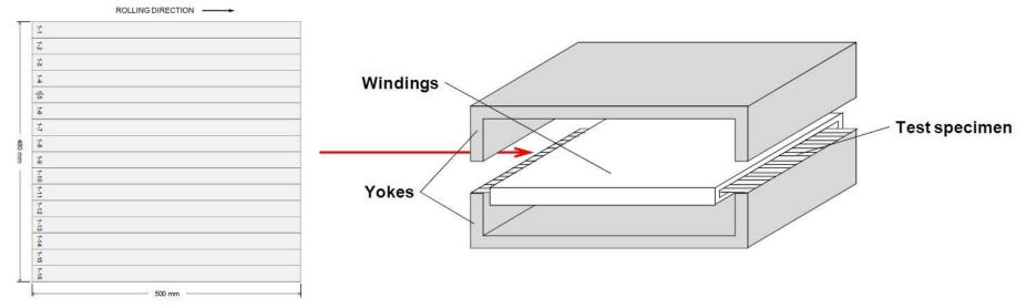
•Strips to be inserted in SST92 apparatus
