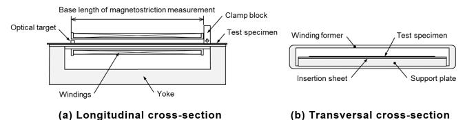
Figure 1 – Schematic diagram of the test apparatus before the improvement
