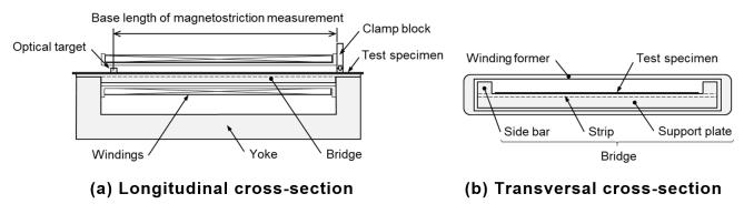
Figure 2 – Schematic diagram of the test apparatus after the improvement
