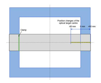
Figure 3 – Range of the positions of the optical target (specified position is -10 mm)
