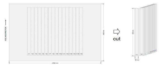
•16 test strips of 500 mm (RD) x 30 mm (TD) shall be cut side by side from a sample sheet of GO materials [3,4]
